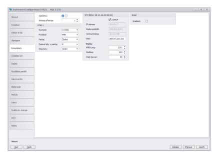
Figure 13: ENVIS.Daq — setting of communication line parameters.
