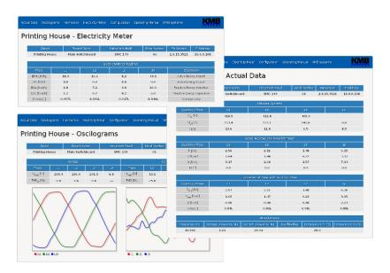
Figure 20: View current data, electricity meter and oscillograms on the instrument's website.
