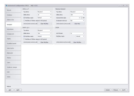
Figure 12: ENVIS.Daq — aggregation setting defines the averaging and evaluation of maximum and minimum values for display and communication.
