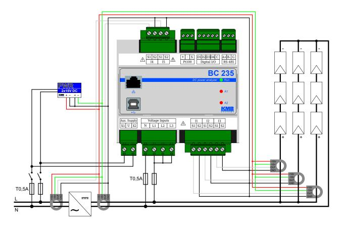
Figure 4: An example of DC voltage, current and power measurement of multiple photovoltaic strings and residual currents before and after the inverter.
