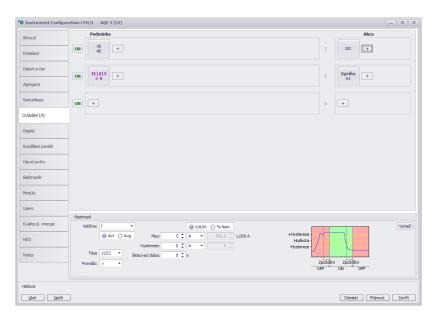
Figure 14: ENVIS.Daq - configuration of programmable inputs and outputs behavior.
