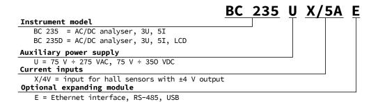
Figure 1: Ordering codes and schemas.
