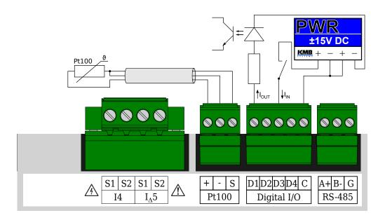
Figure 6: Connection of inputs and outputs in the device BC 235.
