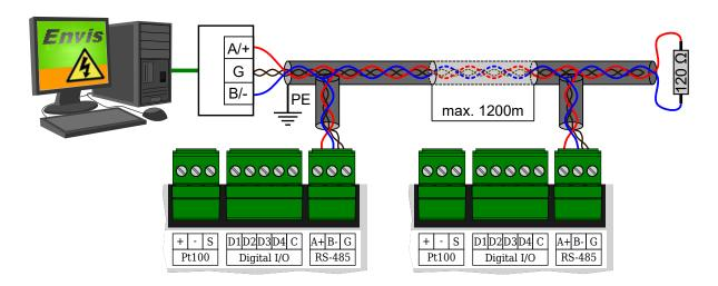
Figure 5: Connection of RS-485 communication lines to BC 235 devices BC 235.
