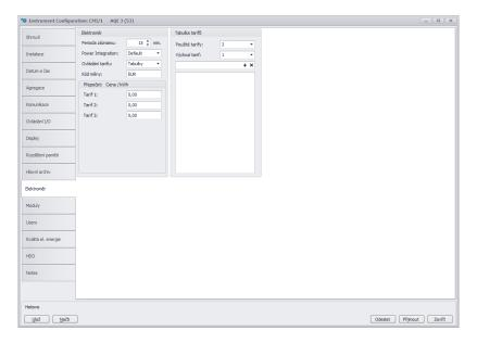
Figure 17: ENVIS.Daq — setting the electricity meter and tariffs and electricity prices.
