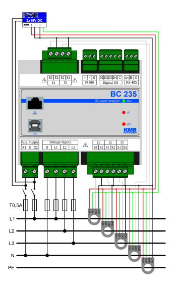
Figure 3: An connection example of BC 235 in a LV AC network with the ability to measure DC components of voltages and currents — "star" voltage measurement in a four-wire network.
