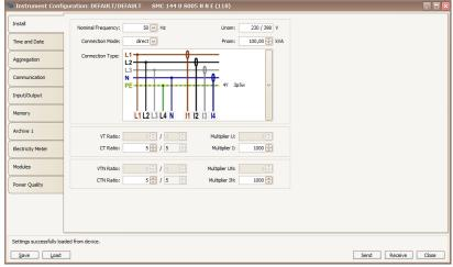
(a) Setting of basic device connection parameters in ENVIS.Daq application.
