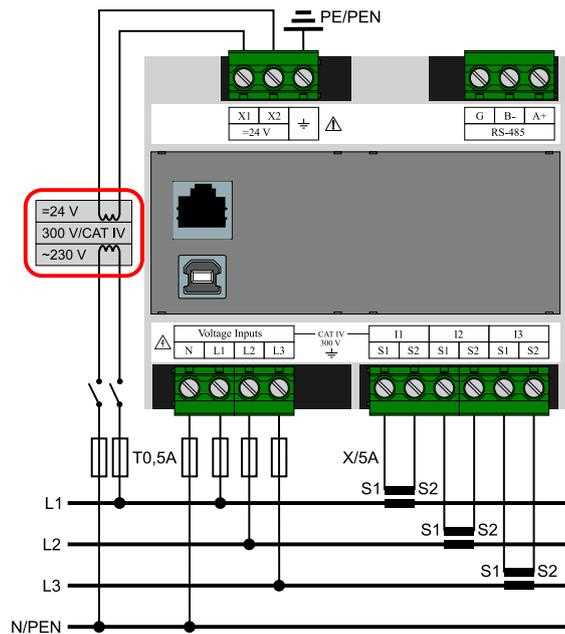
Figure 4: In a 300V/CAT IV network it is necessary to use a power supply with the corresponding overvoltage category! Our PWR1 or PWR3 smart grid power supply is conforming to this requirement.
