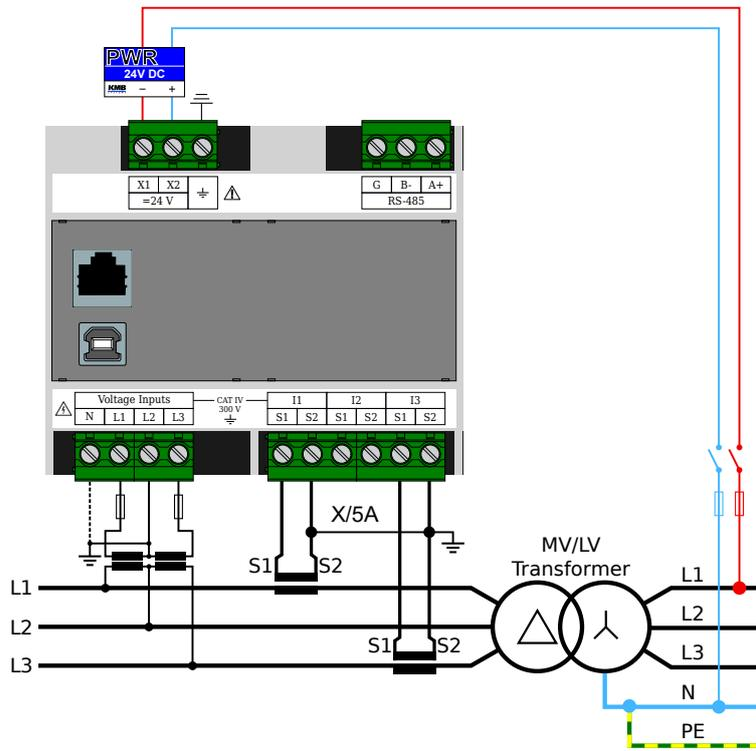
Figure 6: An example of a typical instrumentation of SMC 233 when measured in a MV, HV network on the secondary side of an instrument transformer.
