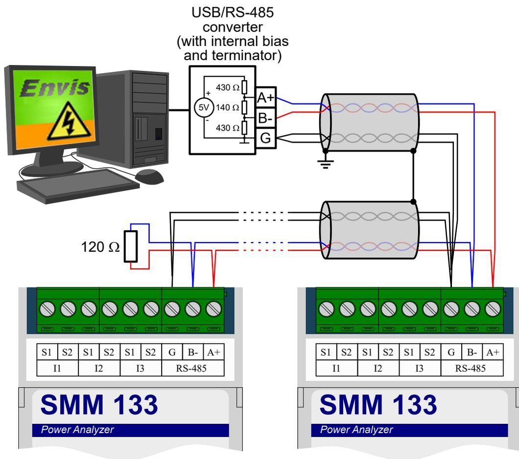
Figure 5: Connection of RS-485 communication lines to SMM 133 devices.
