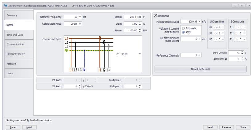
(a) Setting of basic device connection parameters in ENVIS.Daq application.
