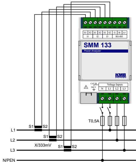
Figure 4: Usual connection of the device in 3p4w network.
