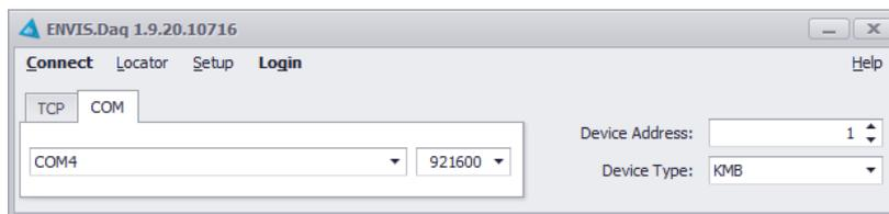
Figure 6: Main window of ENVIS.Daq application after its launch — select the type of communication used, set its parameters and press Connect in menu to continue.
