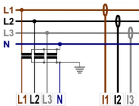
(c) Indirect connection of the device via voltage measuring transformer (in HV, HV networks, etc.).
