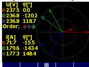
Diagram of actual voltage and current fundamental harmonic phasors.
