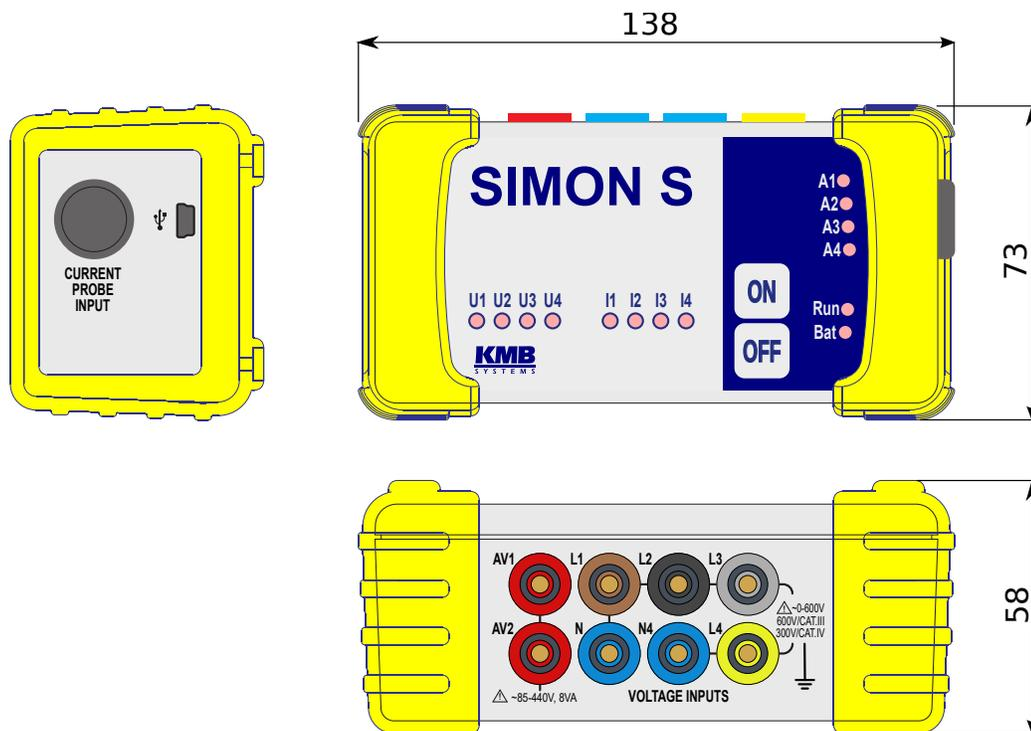
Figure 14: Dimensions of the SIMON S analyzer.
