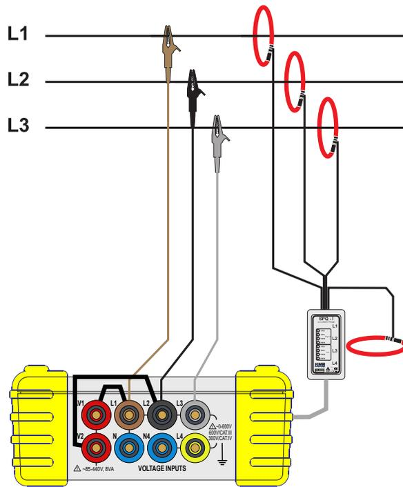
Figure 19: Connection in 3 wire network - supply voltage from line to line voltage via SPQ-Ux jumper
