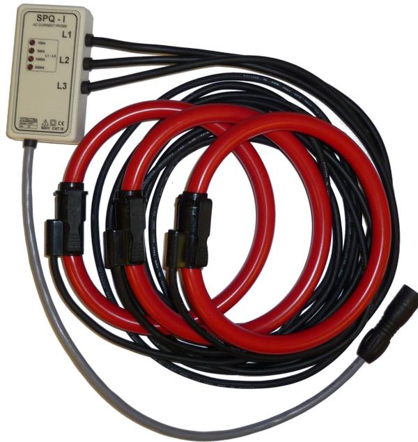
Figure 6: Current probe SPQ-series with three JRF sensors.
