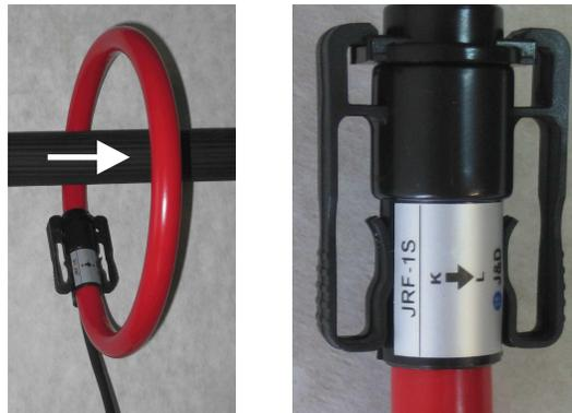
Figure 7: Current probe assembly illustration and detail of current direction indicator.
