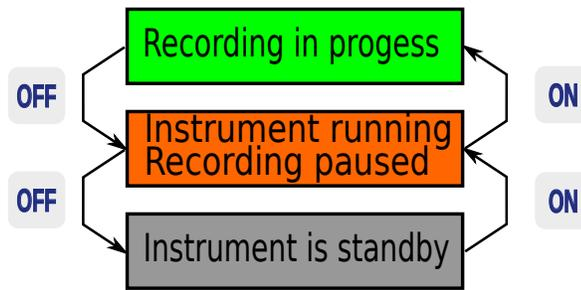
Figure 8: Instrument statuses and function of buttons
