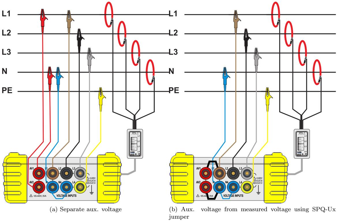
Figure 18: Connection in 5 wire network
