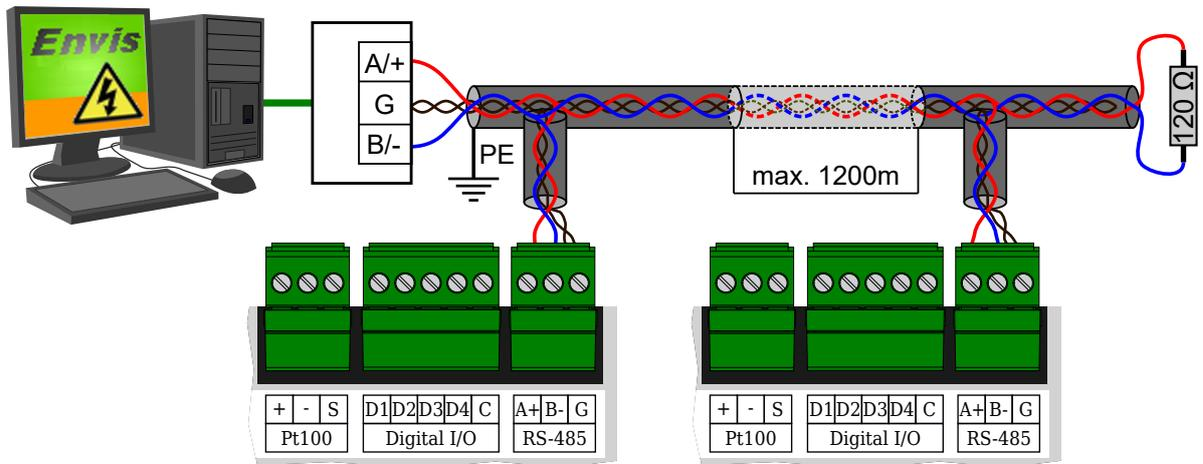
Figure 4: Connection of RS-485 communication lines to MIO 4000 devices MIO 4000.
