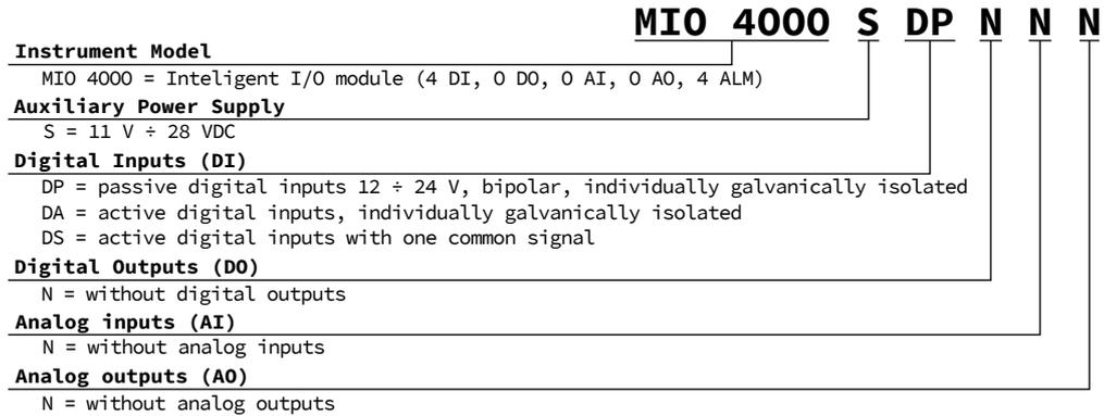
Figure 1: Ordering codes and schemas.
