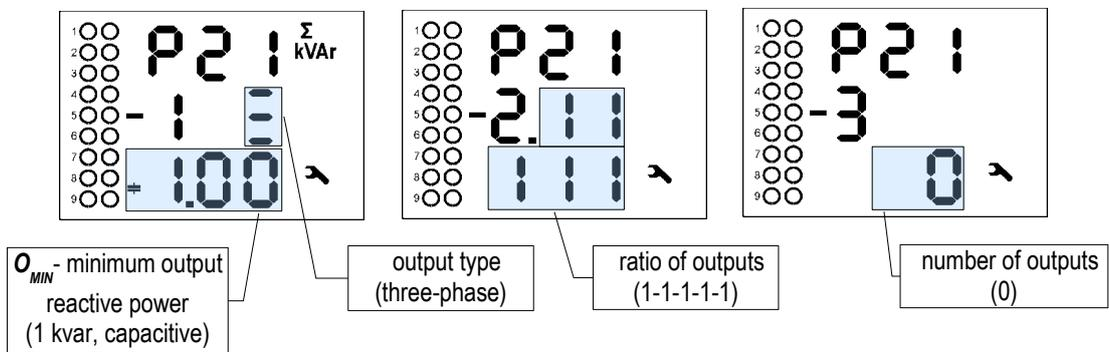
The output type and power presentation is the same as the individual output type & power in the parameter 25 – see below.
