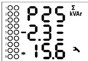
All of the sections' (=outputs') fundamental characteristics are listed at the side branches of parameters 25 ÷ 31.
