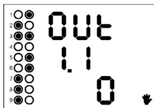
In the first line there is the **OUT** message. With the keys **▲**, **▼** you can scroll through all the outputs (usually from 1.1 to 2.9, the output number in line 2) and check the output actual state in line 3 (0=off, 1=on).
