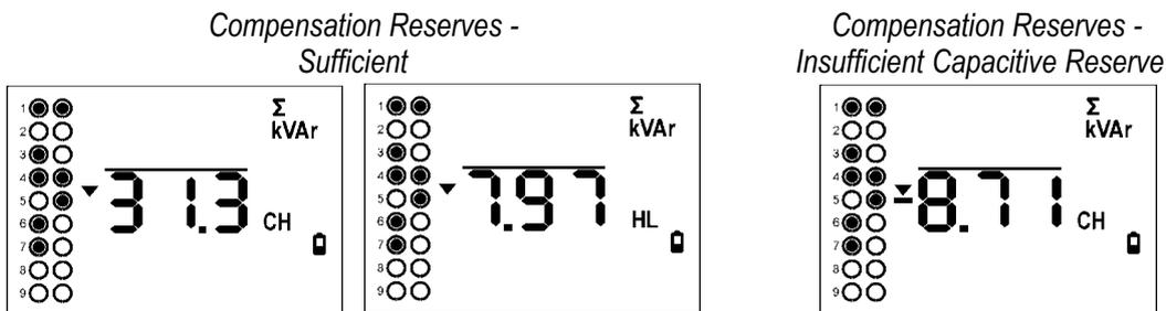
For compensation reactive power capacity assessment, *registered minimum values* of both reserves are decisive. On the left example above, registered minimum of three-phase capacitive reserve is 31.3 kvars, minimum of inductive reserve is 7.97 kvars. As both of them are positive the system compensation power is sufficient.
