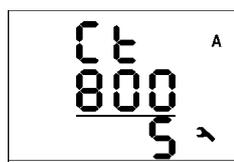
5. line 1 : **C t** - current transformer ratio specification
