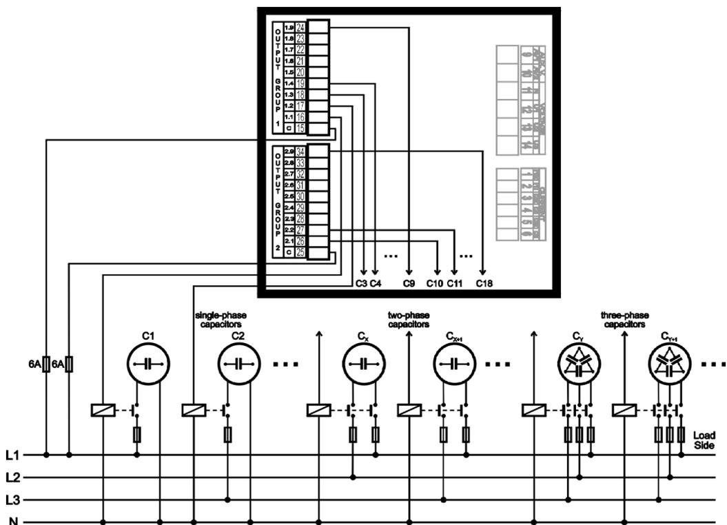
Any combination of compensation capacitors or chokes (three-phase, two-phase or single -phase) can be connected to the instrument outputs via appropriate contactors.
