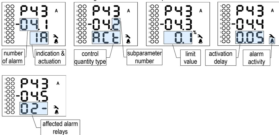
Parameter group No. 43 specifies behaviour of the undercurrent alarm ( mark “I<”). Its number 04 is displayed in the first two characters of line 2. The third character is number of the alarm subparameter :
