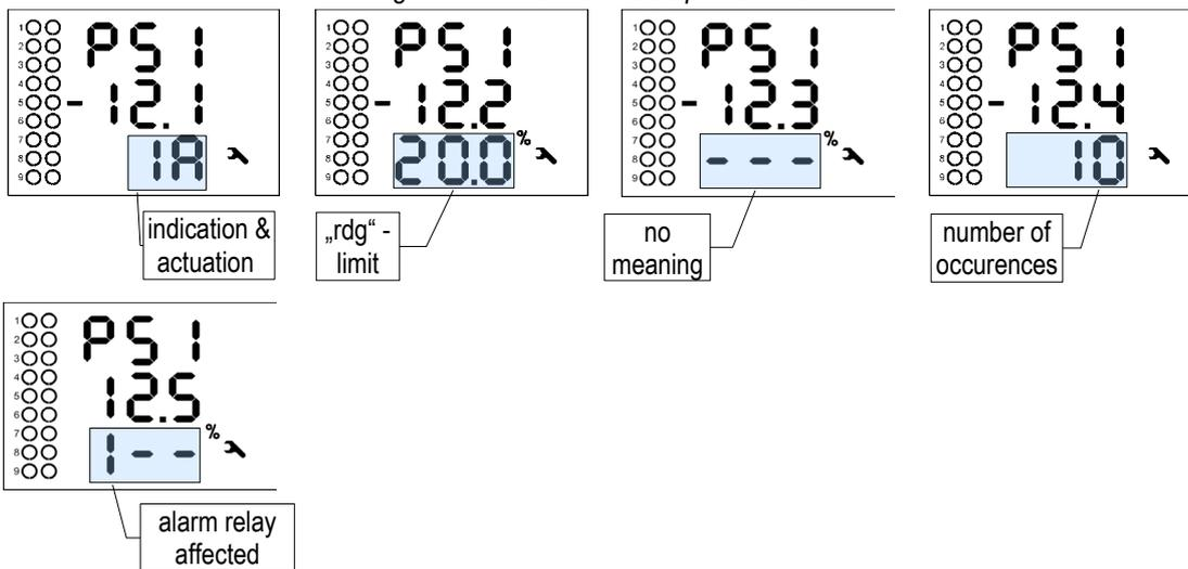
For example, for the alarm setting above, if the three-phase output power is 10 kvars (i.e. corresponding single phase power is 3.33 kvars) the single-phase rdg-component is
