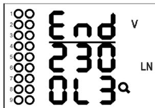
The *End* is shown in the process headline and found U1-angle is displayed in the 3<sup>rd</sup> line (0-L3 in our case).
