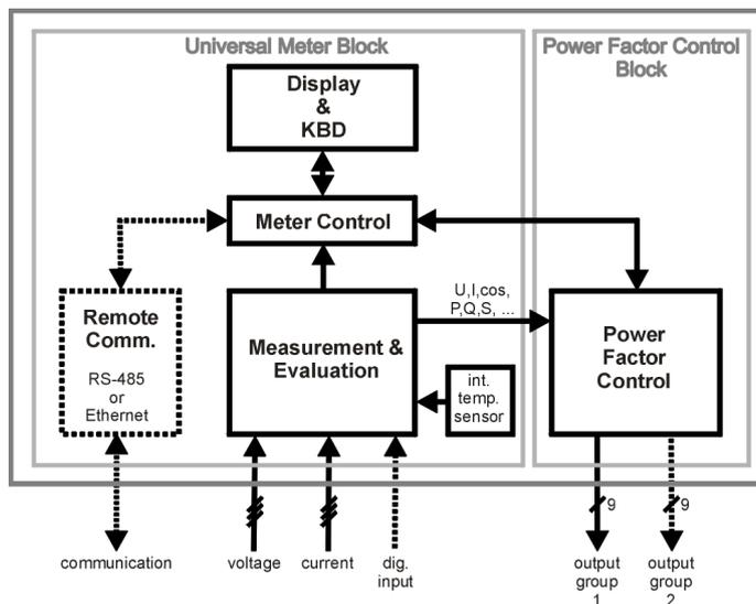
After an activation of supply voltage, the instrument accomplishes internal diagnostics and then it starts to measure and display actual measured data. Simultaneously, the power factor control blocks starts and tries to keep power factor as near as possible to the preset value by connecting optimal combination of compensation elements to the network.
