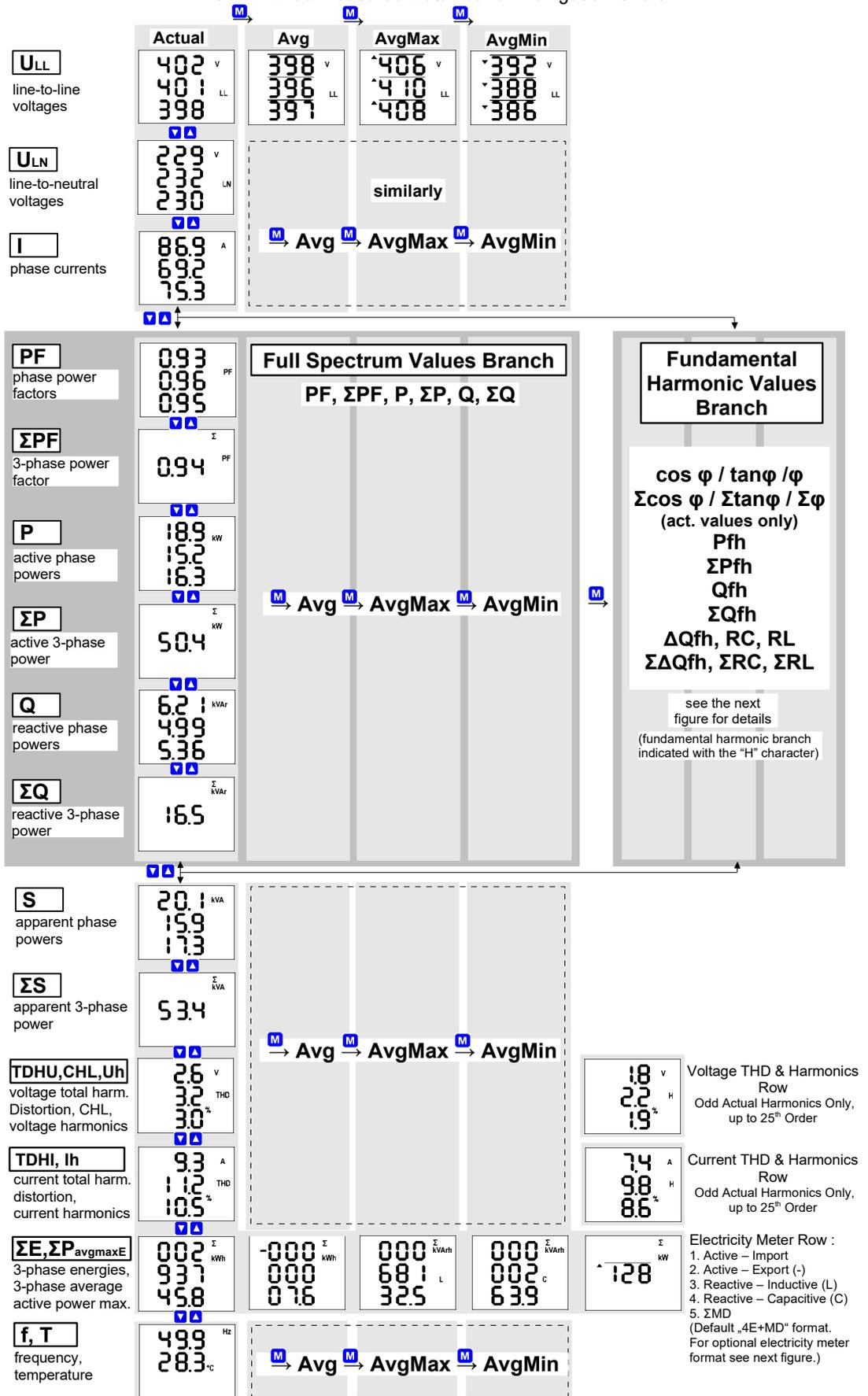
NOVAR 2400 Fundamental Harmonic Measured Values Branch
