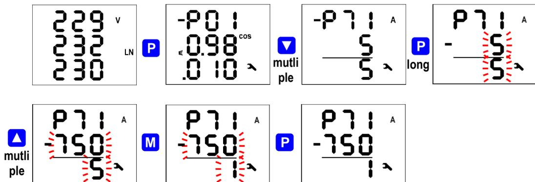
Target CT value is prepared now and we can leave the edit mode with (short) pressing the
