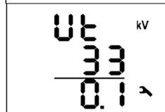
4. when connection of voltage via voltage transformers set (otherwise the screen is skipped) :
