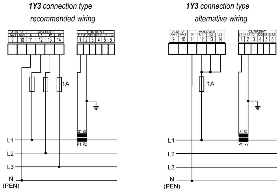
For networks without neutral wire, it is possible to connect all three voltages; then set 1Y3 connection as at previous cases.
