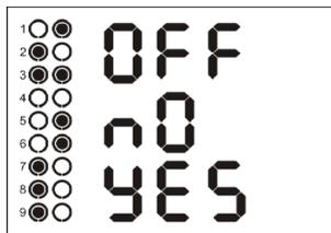
The **OFF** and the outputs that are on flash. Now, with the **▲** and **▼** buttons choose either **No** if you want to keep the output states unchanged, or **Yes** if all of the outputs to be switched off – selected option flashes. Then confirm with **P** or **M**.
