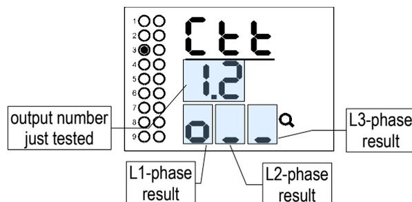
The test can have up to six rounds with four testing steps each. After each step, the measurement results of individual phases are analyzed. If the results of any phase is sufficiently stable, detected current signal connection information is shown in the 3<sup>rd</sup> line, as can be seen in the picture above in the L1 phase result. The connection information can be one of following :
