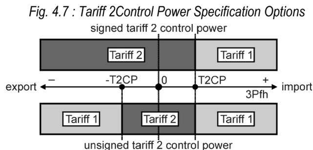
On the contrary, if the *tariff 2 control* parameter is entered with the symbol ▼ only the controller takes it as “**signed**” limit value of power. In such case the tariff 2 parameters applies as soon as positive  $\Sigma P_{fh}$  power drops below the preset level “T2CP” and keeps applied down to zero level and farther to all negative halfplane - see the upper tariff zone bar.
