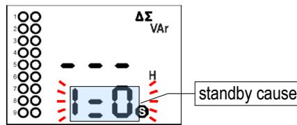
As soon as the events causing the standby state pass the message disappears, standard power factor control process resumes automatically and a control time actual state appears in the line usually.
