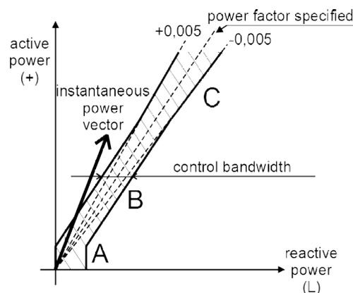
The control bandwidth format is the same as the target power factor. It can be set in range  $0.000 \div 0.040$  if the target power factor format is *cosinus*; if the format is *tangens* or *angle* , the control bandwidth range is  $0.000 \div 0.030$  or  $0 \div 15^\circ$ , respectively.
