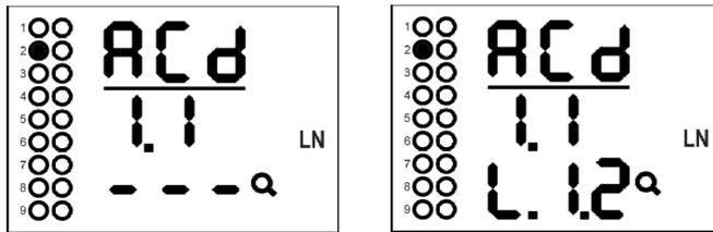
There may be cases where the angle measured with a permissible tolerance does not match any of expected options. Then estimated angle with decimal points appear (right screen).
