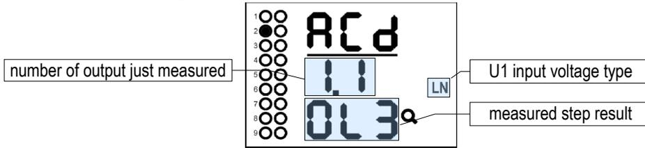
When 1Y3 connection type is set the controller supposes a line-to-neutral voltage (L-N, left screen) is connected; when 1D3 connection type a line-to-line voltage (L-L, right screen) is expected. If unsuccessful step occurs usually dashes appear (left screen below). Such steps are not unusual especially when reactive power in measured network fluctuates strongly.
