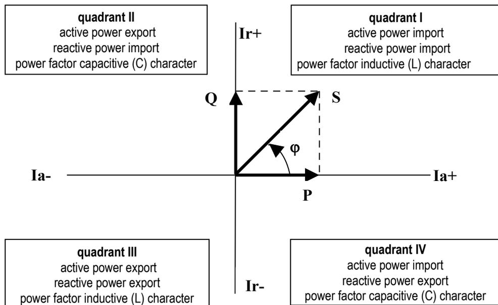
For outright specification of the quadrant, the power factor of the fundamental harmonic component – **cos φ** – is expressed according to the graph with two attributes :
