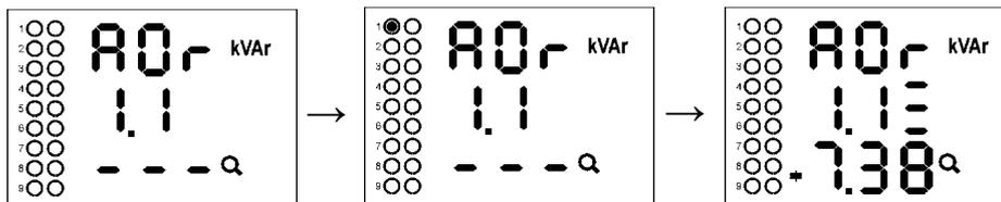
After all of the outputs discharged, the instrument starts to switch the outputs step by step. The number of a step is displayed in the second line and appropriate output is switched on for a short time. After the step is switched off, its type and size is displayed :
