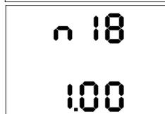
3. line 1 : **n 18** - instrument model (Novar 2400 R18)
