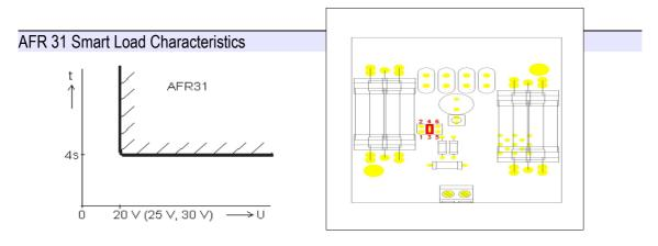
You can set on of three levels according technical parameters table. Default activation voltage level is preset to 25 V. Higher level is suitable for medium voltage grids with higher unbalance of parasitic capacities. After setting, snap in the cover back (keep attention to the correct LED light pipe position).
