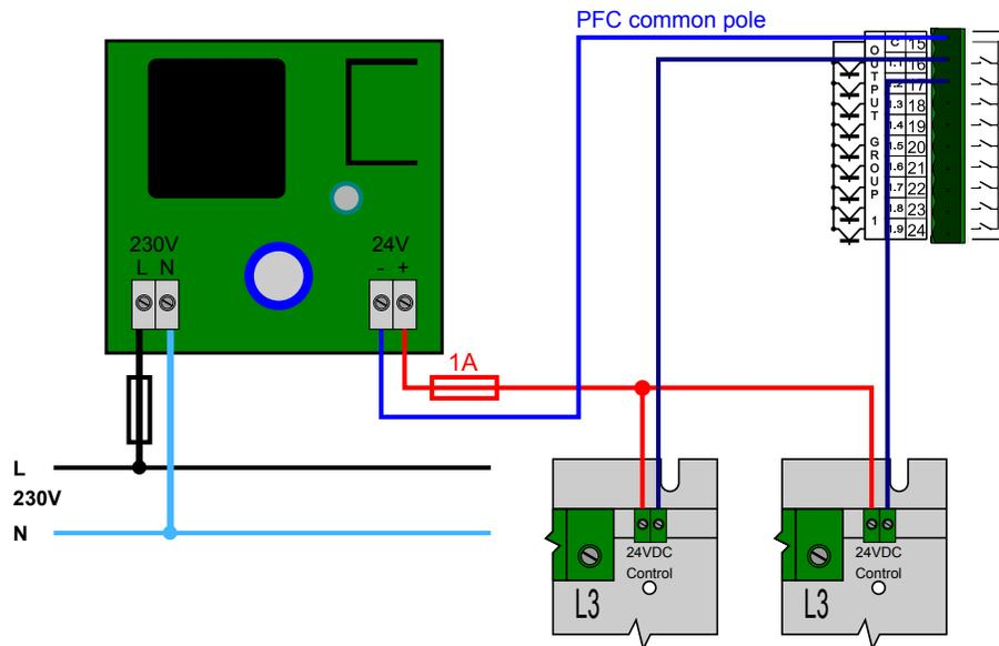
Figure 8: Possible connection of ZP24
