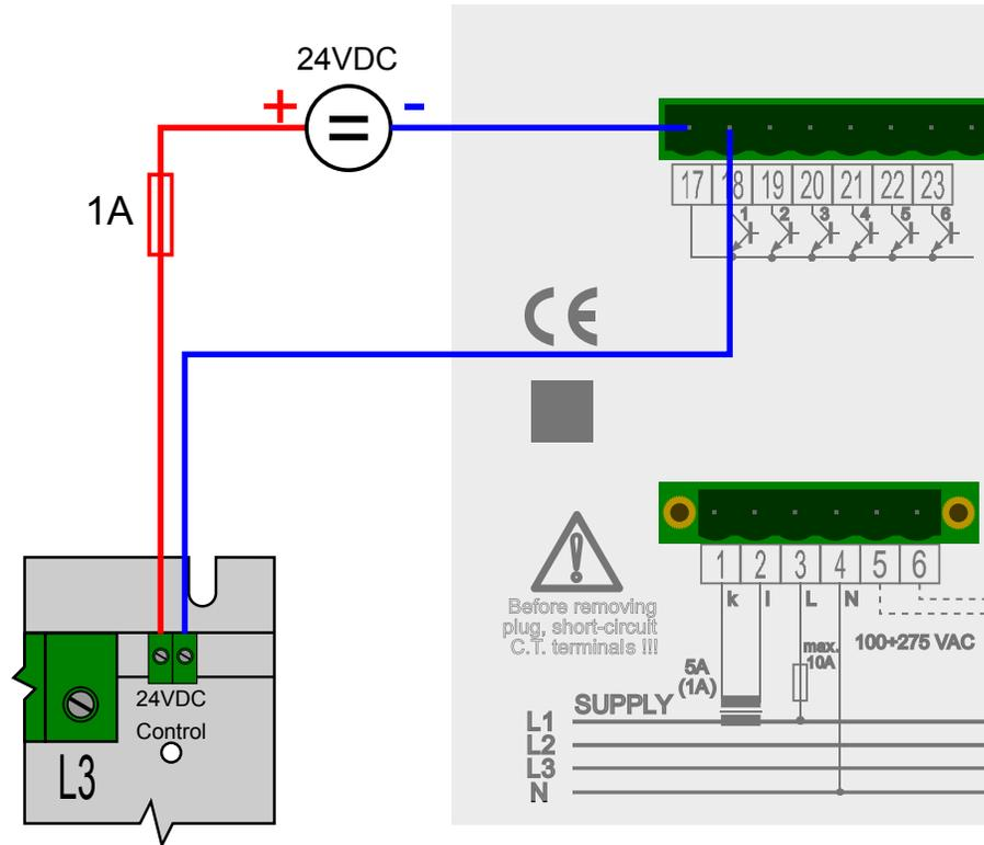
Figure 6: Connection of control signal (polarity-free) to KATKA 20T 400
