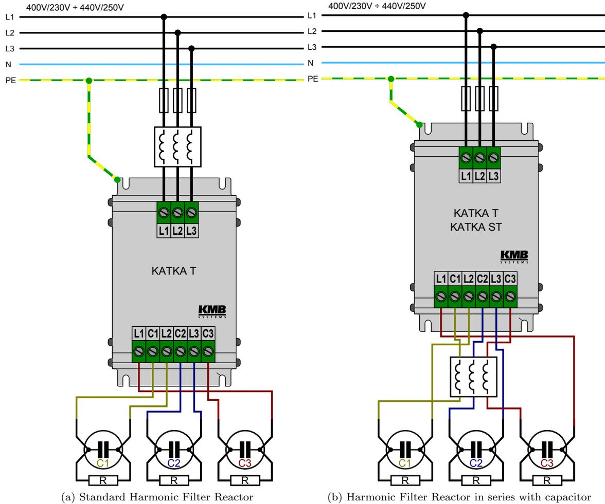
Figure 3: 3 single phase delta connected capacitors
