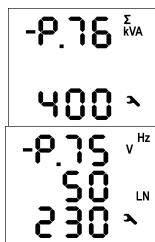
The parameters are arranged in groups, numbered from 00 up. The number of group is displayed in the first line in format - **P. n n** (with preceding dash). You can browse through the parameter groups with the **▲** or **▼** keys.
